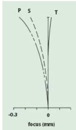
Figure 5b. Illustration of the introduction of negative astigmatism to balance field curvature.
