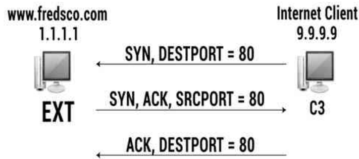
Figure 79.2: TCP Connections and Well-Known Ports
