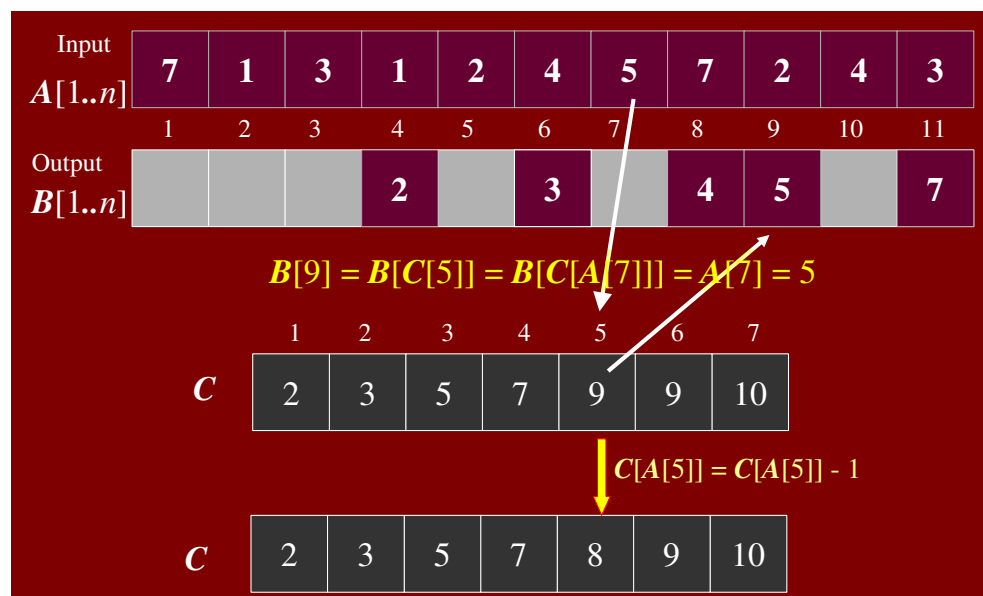
Figure 5.13: A[7] placed in output array B
