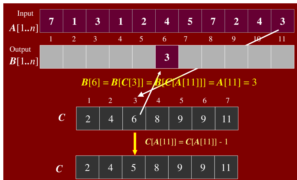
Figure 5.9: A[11] placed in output array B
