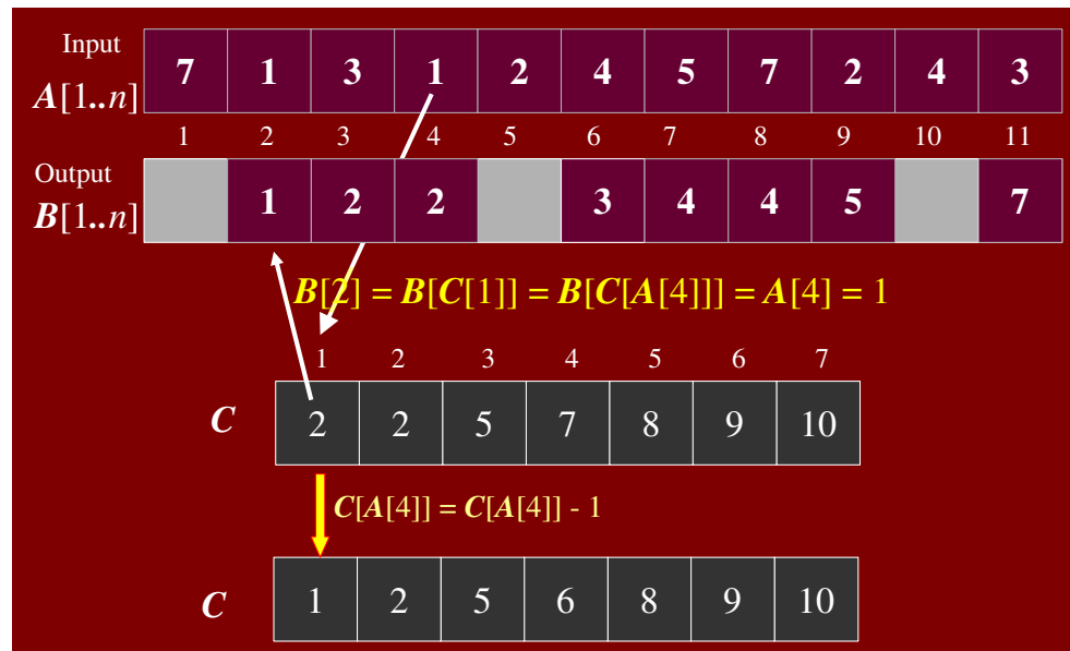
Figure 5.16: A[4] placed in output array B
