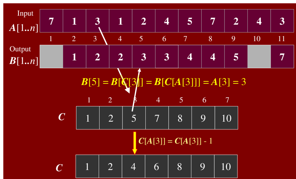
Figure 5.17: A[3] placed in output array B
