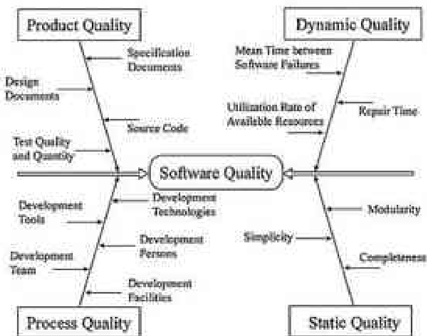
Fig. 1.2 Elements of software quality based on a cause-and-effect diagram
