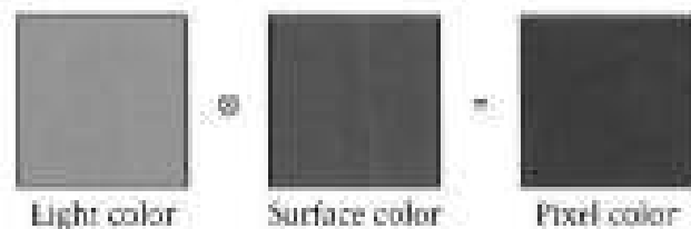
Figure 2: Multiplying (modulating) color values results in a color equal to or less than (darker) the original two.
