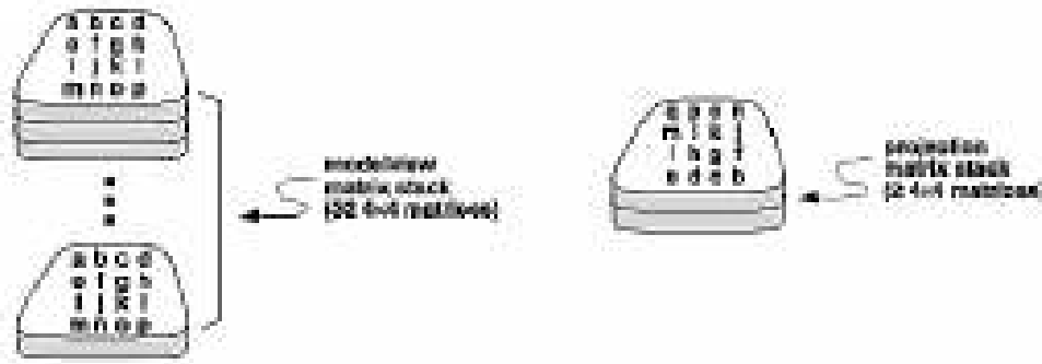
Figure 20 : Modelview and Projection Matrix Stacks
